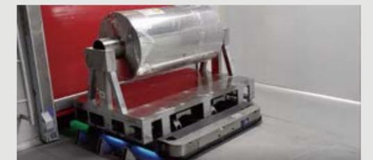
APR Project for Line-side Delivery of Aluminum Shells and Top Covers in a New Energy Company;
